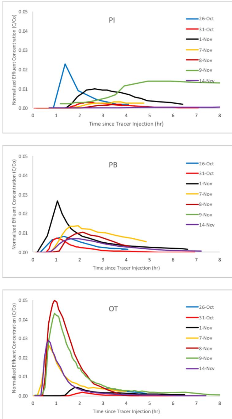
**Figure 3: Tracer breakthrough curves for the first 8 hours after tracer injection at the production interval (PI), below the production interval packer (PB), and at the orthogonal top (OT) monitoring well for the seven tracer tests.**
