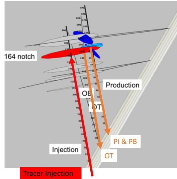
Figure 1: Plan view of the Collab experiment 1 site showing the drift tunnel, and location of the injection well, the 164 notch, and the three tracer sampling locations discussed in this paper.
