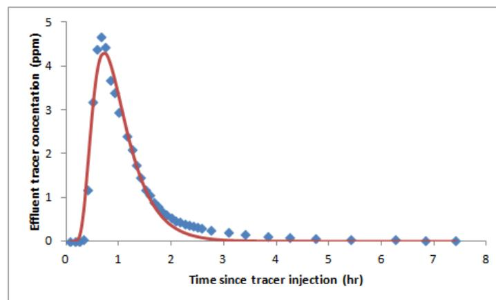
Figure 6: Example of the CXTFIT2 curve fit to the November 14<sup>th</sup> OT tracer breakthrough curve (blue is the sample data, red is the parameter estimation curve fit).
