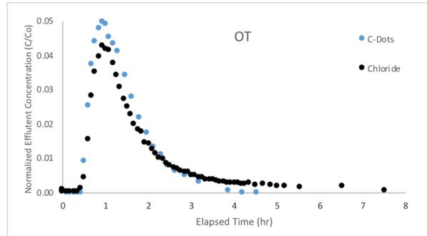
**Figure 2: Comparison of the November 8<sup>th</sup> C-dot (blue) and the November 9<sup>th</sup> chloride (black) tracer breakthrough curves at the OT monitoring well.**
