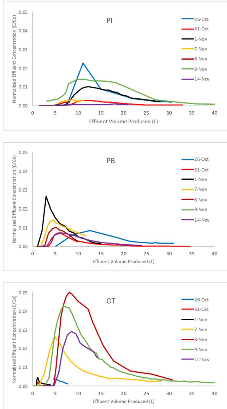
Figure 4: Tracer breakthrough curves as a function of effluent produced at the production interval (PI), below the production interval packer (PB), and at the orthogonal top (OT) monitoring well for the seven tracer tests.
